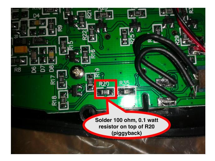
Working with tiny surface-mount resistors with a conventional soldering iron is not simple, but it can be done. I personally recommend getting a strip of these resistors, because I lost a few trying to get one into place for soldering. Note that Danny used a standard through-hole resistor on his microphone mod, which was much easier to solder and achieves the same result.
